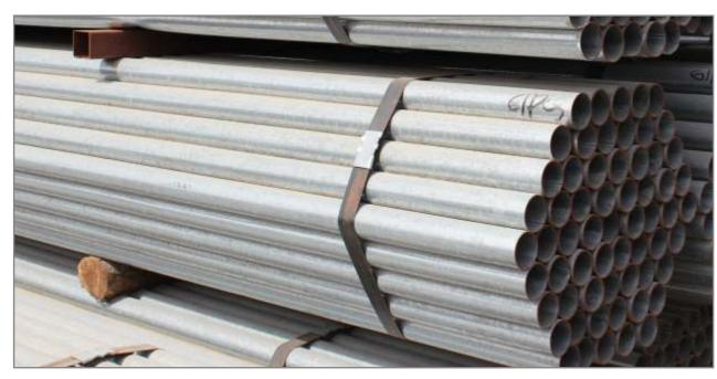
SIZE RANGE FOR GALVANIZED PIPES: 1/2" TO 8" THICKNESS RANGE FROM: 1.0MM TO 6.0MM
